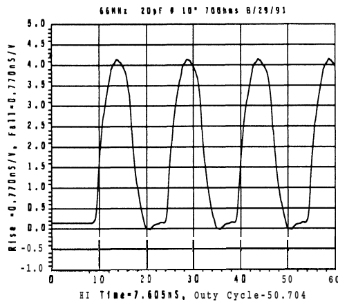
20 pF Load with 10" of Trace (Zo=70Ω) Single Driver
